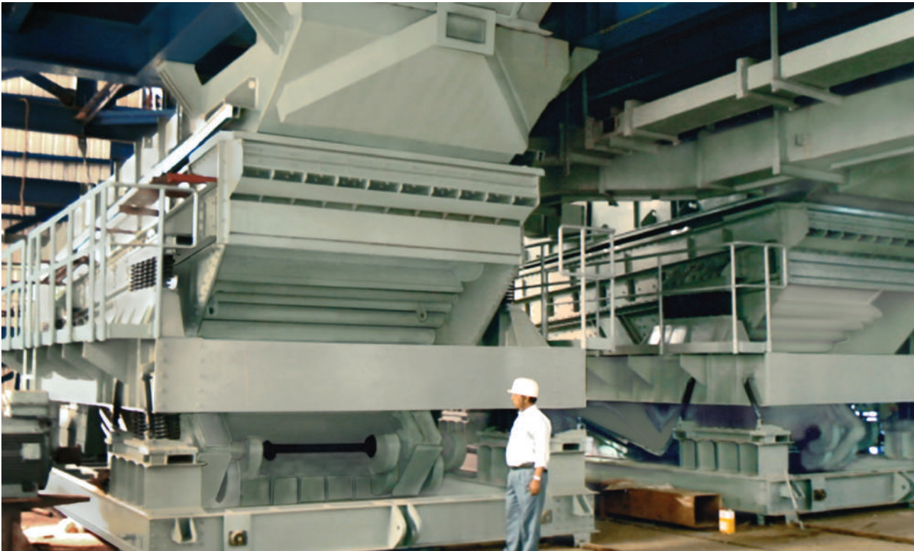
3.1m x 8.5m Linear Motion Screen on Isolation Frame and Trolley - Screening Sinter
