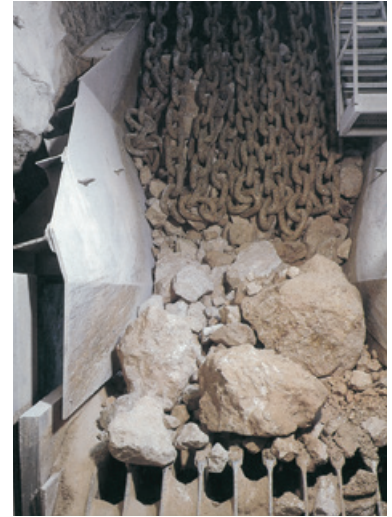
Grizzly Screen Feeder handling up to 2.0m material lumps
