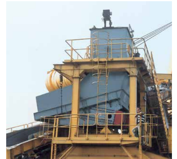
Mechanical Vibrating Feeder 2.5 x 7.0 m
