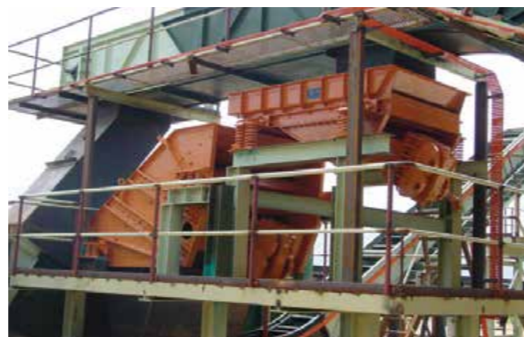
Linear Motion Feeder with Vibro Bar Sizer
