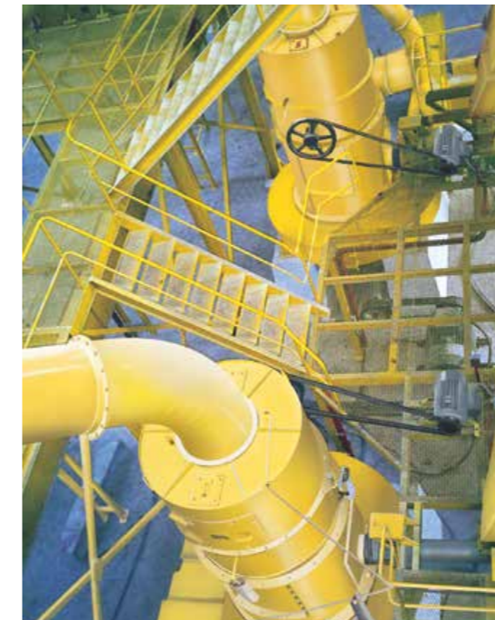
Roller Mills Grinding Barite
