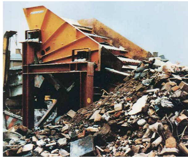
VIBRO-BARSIZER handling upto 800 mm feed size
